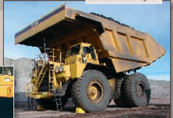
Caterpillar 793 Haul Truck (240 ton) chocked using two Model 1911 Monster Wheel Chocks.
